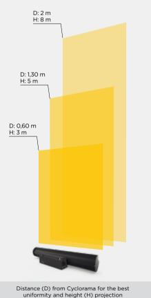
uniformity and height (H) projection Minimum recommended distance: 0,60 m Maximum recommended distance: 2 m
